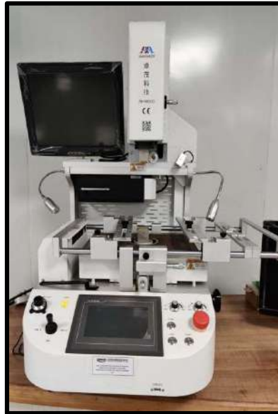
BGA Rework Station
